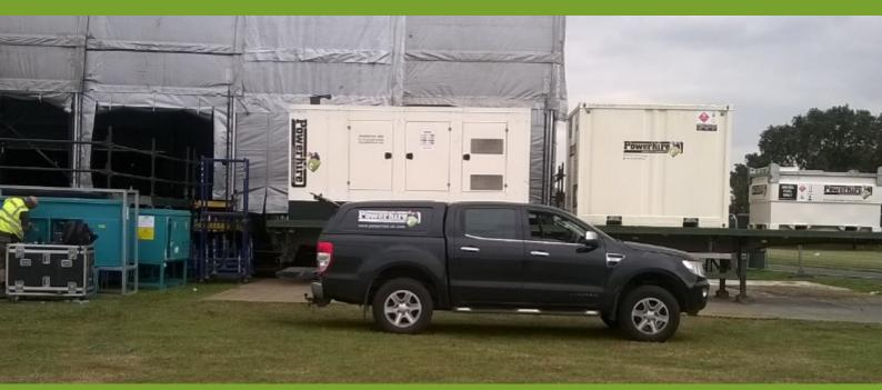
In collaboration with the organisers Powerhire's Engineers safely delivered and positioned their twenty+ generator sets and fuel tanks four days prior to the commencement of the event. They specified their super silent event spec ready generator sets ranging from 20kVA up to 500kVA synchronised units totalling a complete power package of 3.5 MVA, together with supplying bulk fuel storage units ranging from 3000 up to 8000 Ltr fully bunded containerised tanks.
